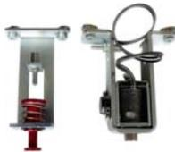
Blocking device that consists of a monostable electromagnet with a pin to block the leaves displacement cart. It includes a manual device to unblock the door from the inside.
